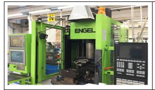
ATAM\_Presses for thermosetting epoxy resin overmoulding, inserted in the IoT system of the company.
