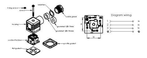
The connector is supplied with a set of two NBR sealing rings (cable gland) for cables with a sheath diameter between 5 and 7mm or between 8 and 10mm, and two NBR sealing rings with the counterpart (one optional to the other).
