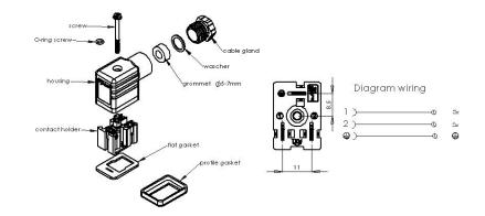
The connector is supplied with a set of two NBR sealing rings (cable gland) for cables with a sheath diameter between 5 and 7mm, and two NBR sealing rings with the counterpart (one optional to the other). During installation, the correct assembly and integrity of all the parts must be verified.
