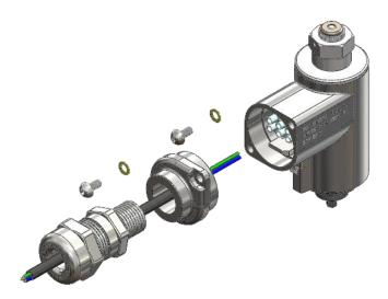
**Step\_3**Remove the connector and then proceed with main wiring to the proper positions as indicated below according to voltage type (AC or DC).
